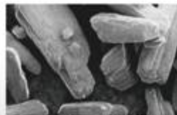
針状結晶が集積した原薬粒子 (流動不良や二次凝集の原因) API crystals have long and thin shapes (Cause of poor flowability or secondary agglomeration)
