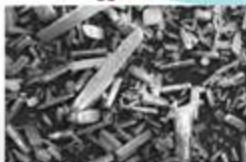
針状結晶が集積した原薬粒子 (流動不良や二次凝集の原因) API crystals have long and thin shapes (Cause of poor flowability or secondary agglomeration)
